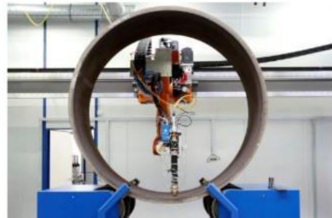
Diode Laser Cladding equipment setup (images courtesy of NAMRC)
